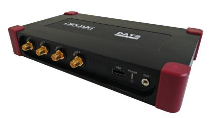
The DATS-solo is a pocket-sized, ultra portable, high quality, 24-bit data acquisition system. It is compact, rugged and has 4 inputs selectable as IEPE, voltage or tachometer inputs. Industry standard SMA connectors are used for input with optional adapters for other connectors. The size, tough packaging and power from USB make it ideal for mobile use. Internally there is comprehensive signal conditioning for IEPE or voltage with anti-alias filters, all controlled by Prosig's DATS software.
