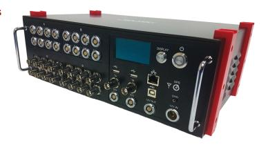
The DATS-tetrad is a rugged, portable data acquisition system that supports up to 32 high speed analog inputs and can be stacked for higher channel counts. Many sensor input options are available including microphones, accelerometers, strain gauges, thermocouples, load/pressure/force sensors, tachometers, rotary encoders, digital I/O and CAN-bus. Analog output and digital output are available with options for open and closed loop control. The system has an optional internal GPS receiver.
