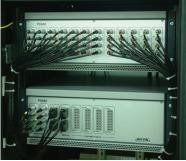
There are 112 analogue inputs in total plus 32 thermocouple inputs, CAN input and digital lines.
