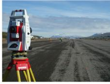
programme was undertaken to study the displacement of the road surface as a vehide passes over. The objective of the study was to understand the behaviour of the pavement. Using the results, the construction of future pavement could be improved and maintenance costs reduced.
