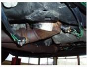
Supplied with cooling water via a windscreen washer pump, the accelerometer cables and cooling
