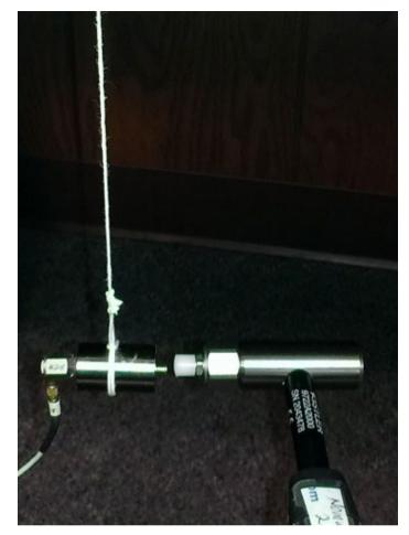
Figure 2: Improvised system to calibrate an impact hammer
